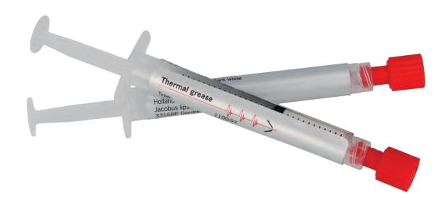
Thermal grease is a ceramic-filled single-component silicone with high thermal conductivity. The non-cross linked thermal compounds will not dry out and the silicone components do not leak out of the compound. The silicone-free thermal compound 1100-12 consists of synthetic, thermal polymer and is suitable for fast and effective heat dissipation.
