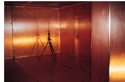
Mu-copper Faraday cage, Mu-copper wall covering system
