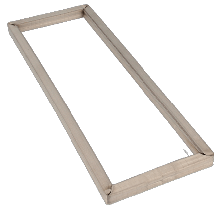
8100 series Frame gasket example. Version with conductive textile and low closure force polyurethane foam.
