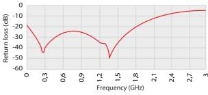
3 mm thick ferrite tile + 21 mm gab + 3 mm thick ferrite tile
