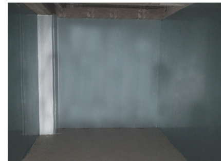
Aluminium foil to create a Faraday cage
