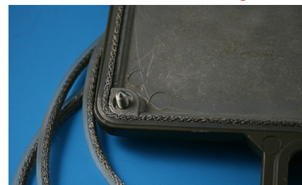
Metal knit EMI/RFI gasket in a groove
