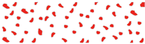
Contact points of metal knit gasket
