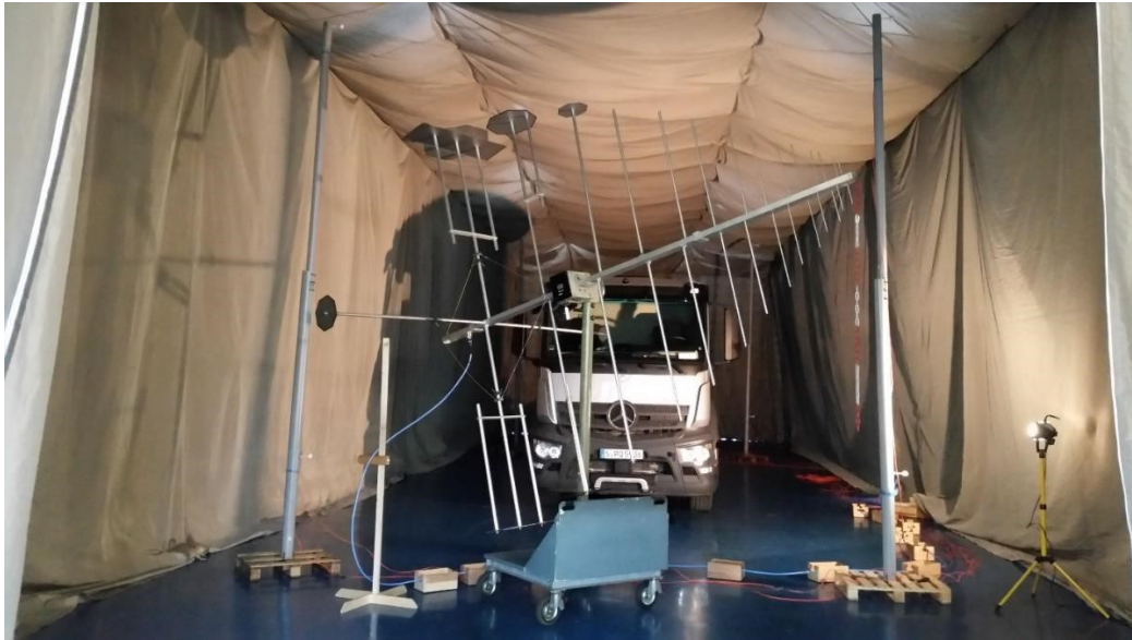
Figure 2: Truck in the test field defined test volume within the columns is irradiated with a LogPer antenna.
