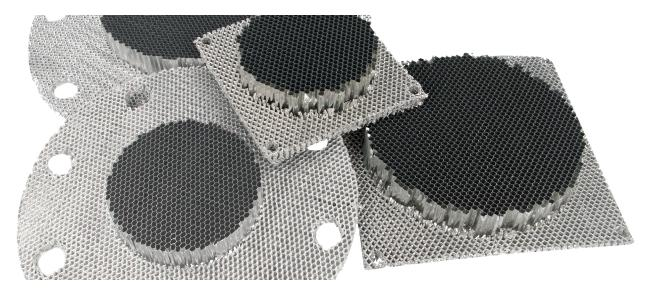
Honeycomb vents are used to EMI shield openings for ventilation or acoustic/visual contact. We can make these vents according to your drawing within a few days, or you can use our standard range from stock. Honeycombs are also frequently used as flow straighteners to create a laminar flow.
